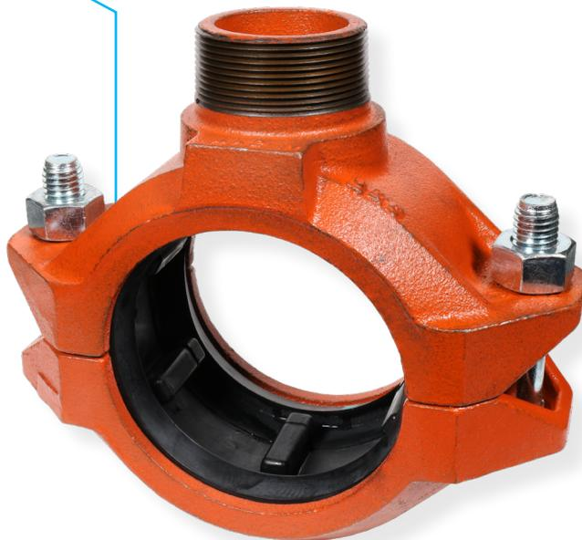
The Gruvlok Fig. 7042 Outlet Coupling is designed to join two sections of grooved end pipe and form a reducing outlet connection. The outlet couplings are available for the 1½" through 6" IPS or ISO run pipe sizes with the outlet pipe sizes ranging from ½" through 2".
